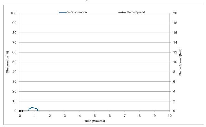
Test Num.: 1 NC / 4791550635 NTN12182404 Flame Spread Index: 0 Smoke Developed Index: 0 Max. Flame Spread (ft.): 0.0
